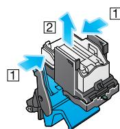
7 Attach a new staple case to the **Saddle Staple Cartridge**.
