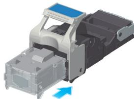
→ Insert the staple case until it hits the back of the **Staple Cartridge**, and check that it is locked.
