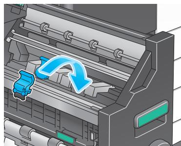
**10** Push the blue knob of the **Saddle Staple Cartridge** to the back.
