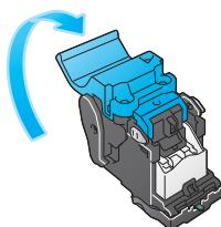
**9** Attach the **Saddle Staple Cartridge**.
