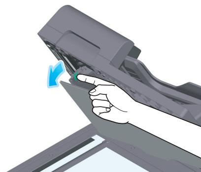
→ Release the lock lever of the **Opening and Closing Guide**, and open the **Opening and Closing Guide**.
