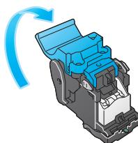
9 Attach the **Saddle Staple Cartridge**.
