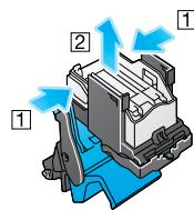
7 Attach a new staple case to the **Saddle Staple Cartridge**.
