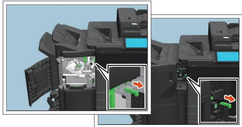
3 | Pull the lever to unlock the finisher.
