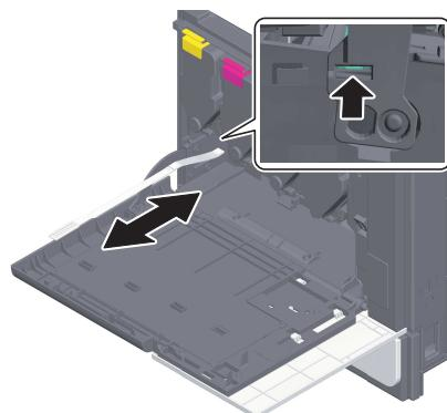
**5 Mount the **Printhead Cleaner** onto the **Front Door** of this machine.**
